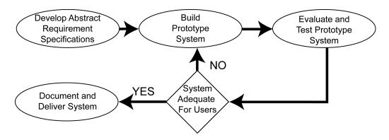
Figure 2. Evolutionary prototyping
