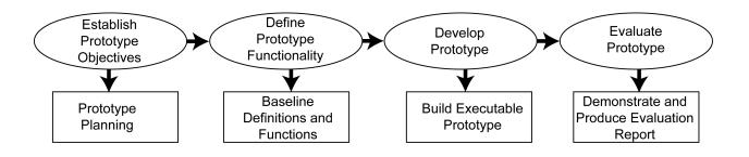
Figure 1. Process Model for Prototype Development
