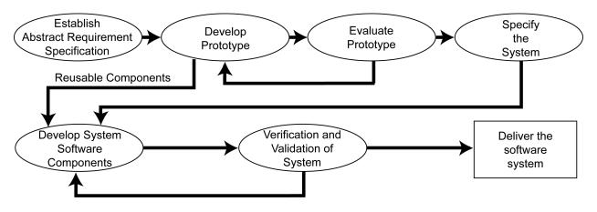
Figure 3 Throwaway prototyping
