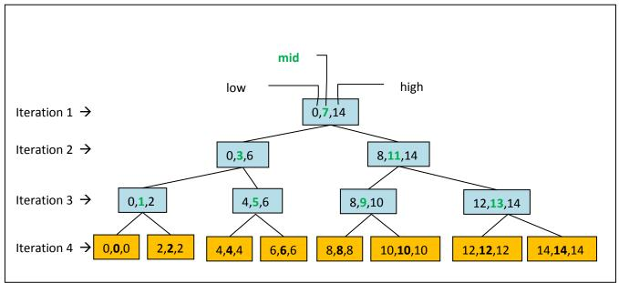
Figure 2. A binary tree showing the number of iterations for each element in an array of 15 to be found via binary search
