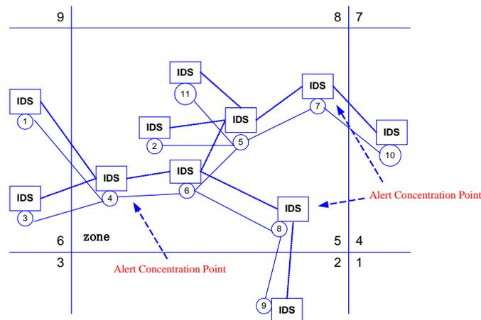
Fig. 1. The Zone-Based Intrusion Detection System (ZBIDS) for MANETs.
