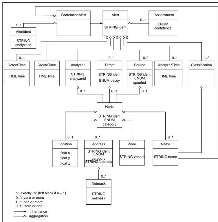
Fig. 5. MANET Intrusion Detection Message Exchange Format (MIDMEF).
