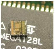
Photo courtesy <u>JLH Labs</u> "Spec" sitting on top of the previous generation of UC Berkeley Motes, the Mica node. The size reduction is amazing.
