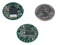
Photo courtesy <u>Crossbow Technology</u>, Inc. The MICA2DOT mote, typically powered by a circular "button"
