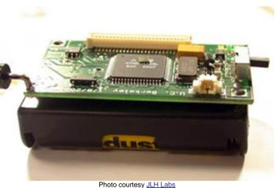
Broad view of "Spec" sitting on top of the previous generation of UC Berkeley Motes, the Mica node. "Spec" is the tiny little square on top of the raised bit in the middle.
